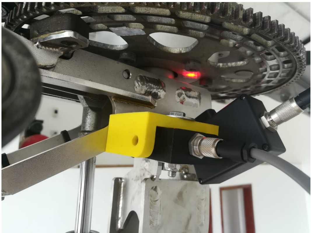
Fig 3.2. Sensors mounted on an MTO rotor head (rear-right view)
