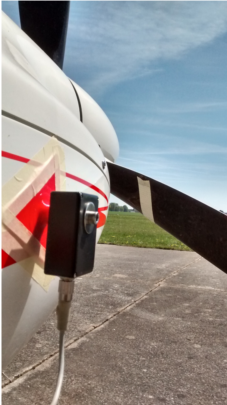
Fig 2.4. Tacho sensor mounted on cowling
