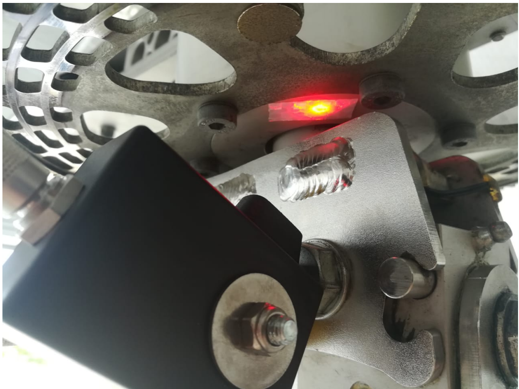
Fig 3.8. Tacho shining onto reflective tape attached to prerotator disk
